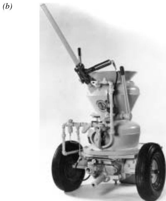
Fig. 3.1—(a) Schematic of a double-chamber gun (dry process); and (b) double-chamber gun (dry process).
